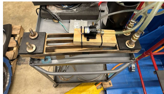
Fig. 5. Keel cooler used for the OSTEC PTO cooling system.
