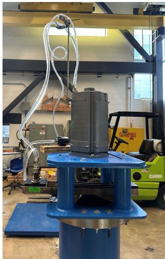
Fig. 7. Siemens 26.2 kW permanent magnet servo drive installed on the custom build test stand for OSTEC turbine.
