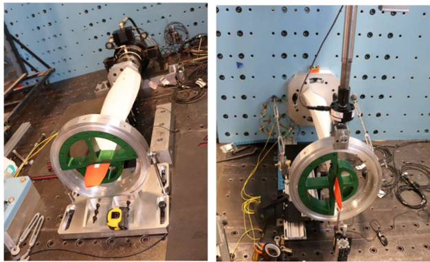
Fig. 11. Bending moment and torsion testing of blades
