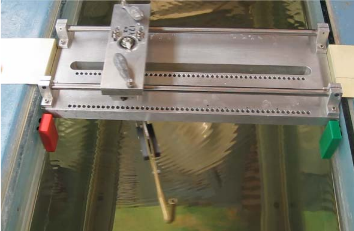
Figure 13. The oscillator with magnets for flat plate reversal and weights attached.
