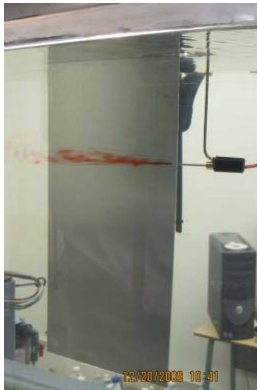
Figure 24. Initial flow separation of dye stream.
