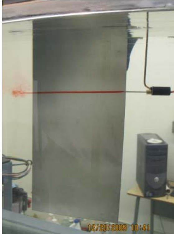
Figure 22. Attached laminar dye stream.
