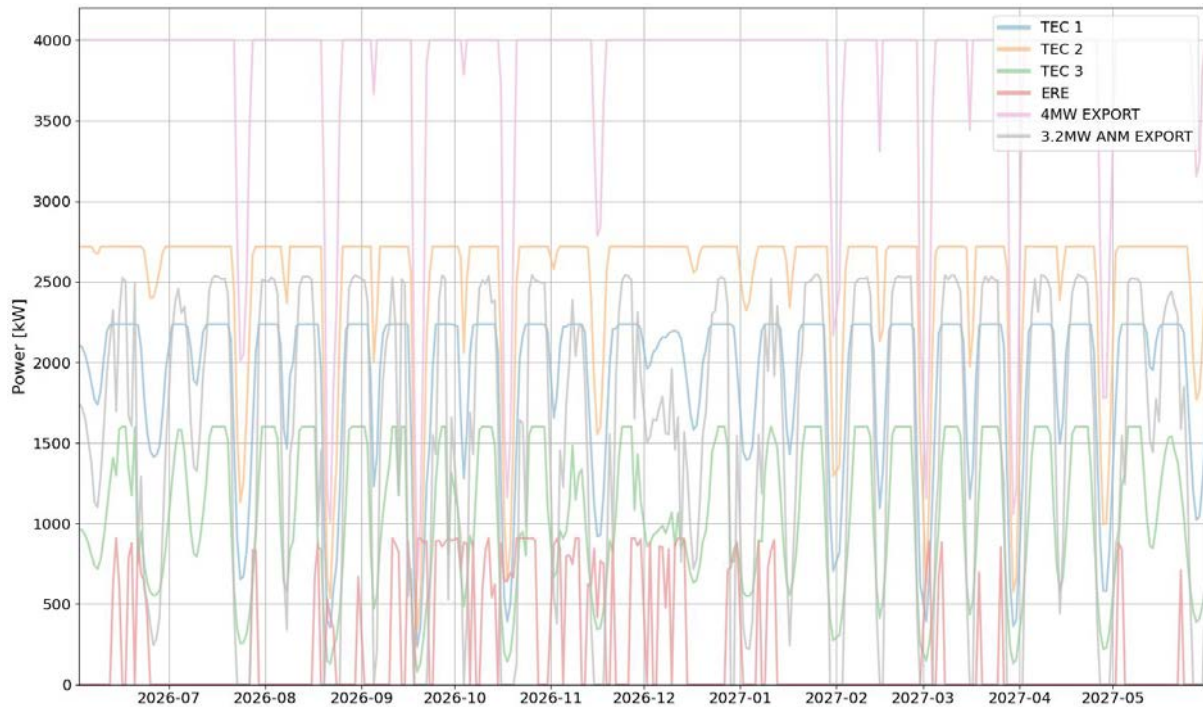
Figure 3 | Generator and site daily maximum export power [kW] June 2026 – May 2027
