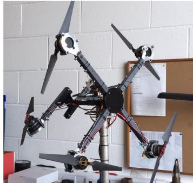
Fig 3. Multi-Propellor Device (MPD) developed to simulate aerodynamic loads using fans 3
