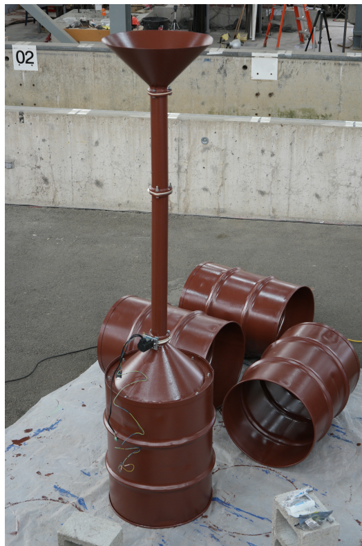
(a) Photo of OWCs being built
