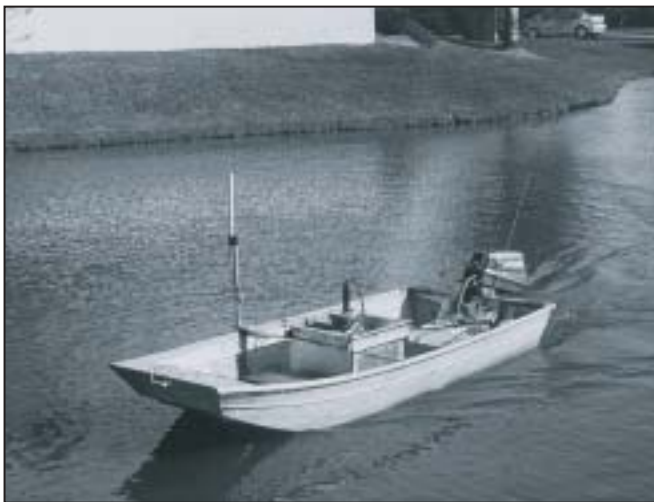
Figure 4.7. Radio-controlled, 12-foot, broad-band acoustic Doppler current profiler platform.
