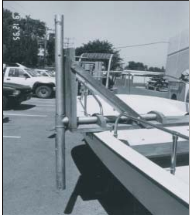
Figure 4.14. Inexpensive acoustic Doppler current profiler mount.
