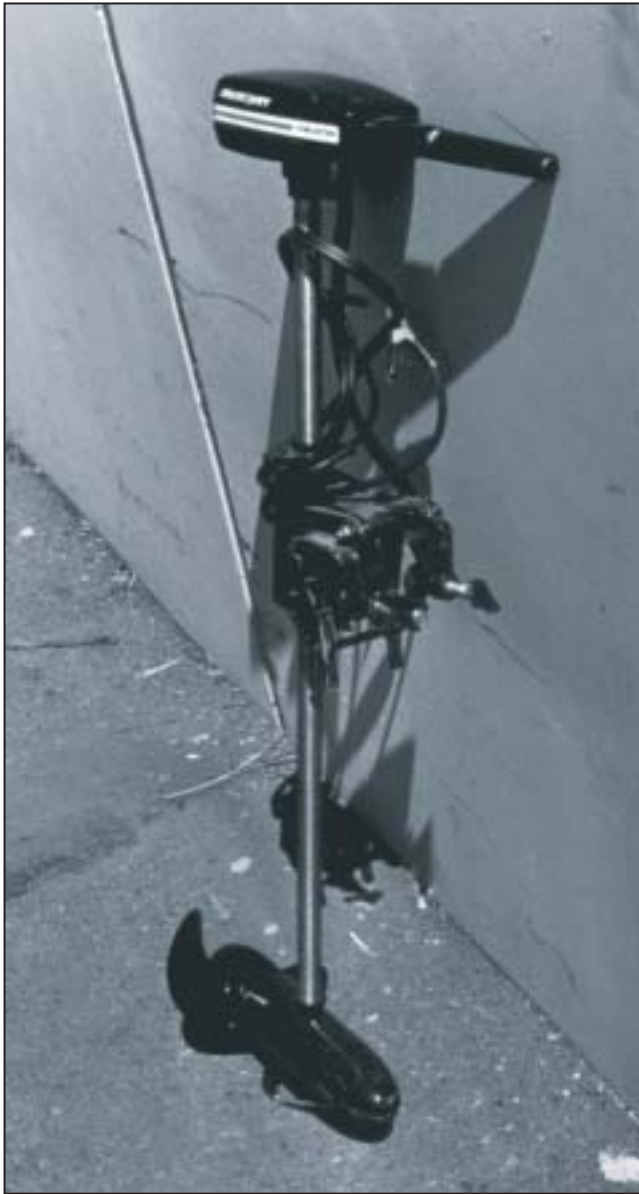
Figure 4.23. Typical battery-operated trolling motor used when making acoustic Doppler current profiler discharge measurements.
