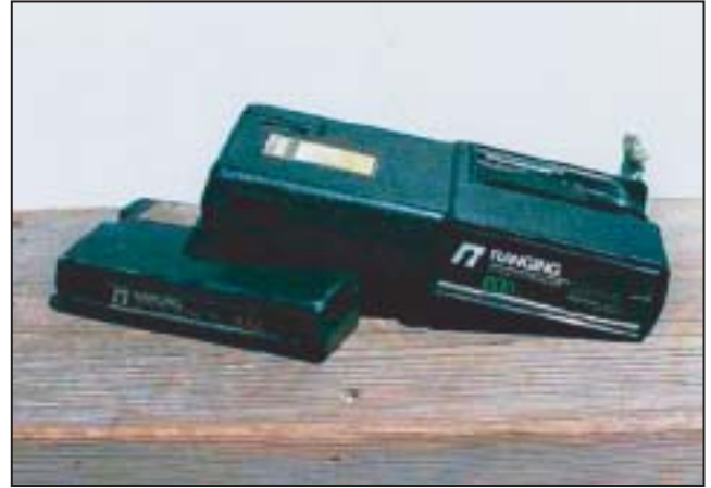
Figure 4.22. Optical range finders used to estimate near-shore distances.
