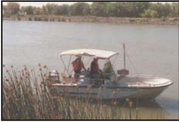
Figure 7.5. Acoustic Doppler current profiler vessel at the beginning of a discharge measurement.
