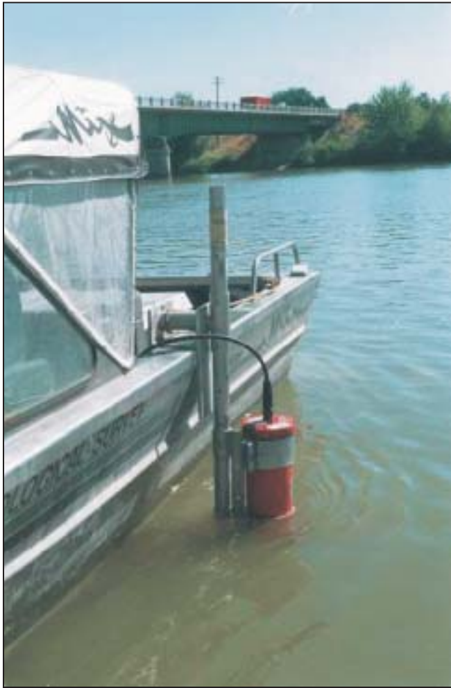
Figure 4.21. Detachable swing mount used by the U.S. Geological Survey Idaho District.
