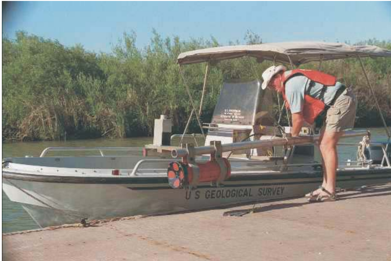
Figure 4.9. Side-swing mount on a 6-meter (20-foot) Boston Whaler for an acoustic Doppler current profiler.
