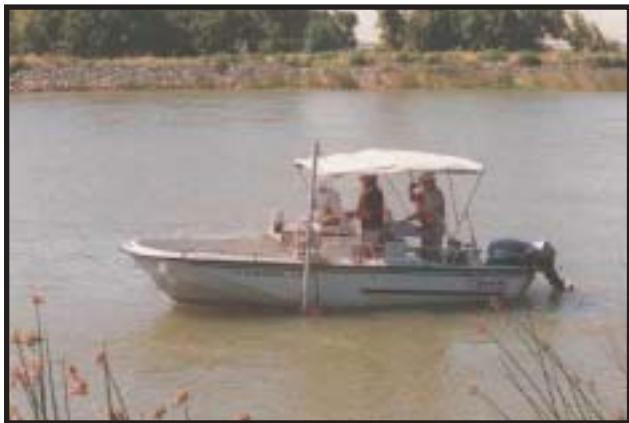
Figure 7.7. Acoustic Doppler current profiler vessel at the end of a cross-section traverse.
