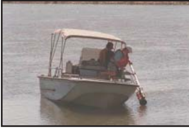
Figure 7.3. Broad-band acoustic Doppler current profiler mount being deployed vertically.
