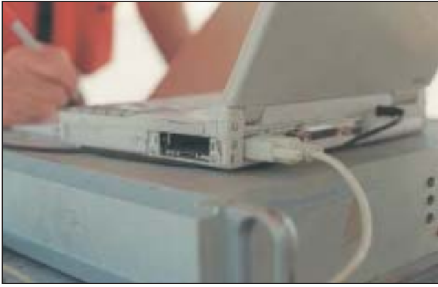
Figure 4.13. Laptop computer with missing plastic doors and port covers.
