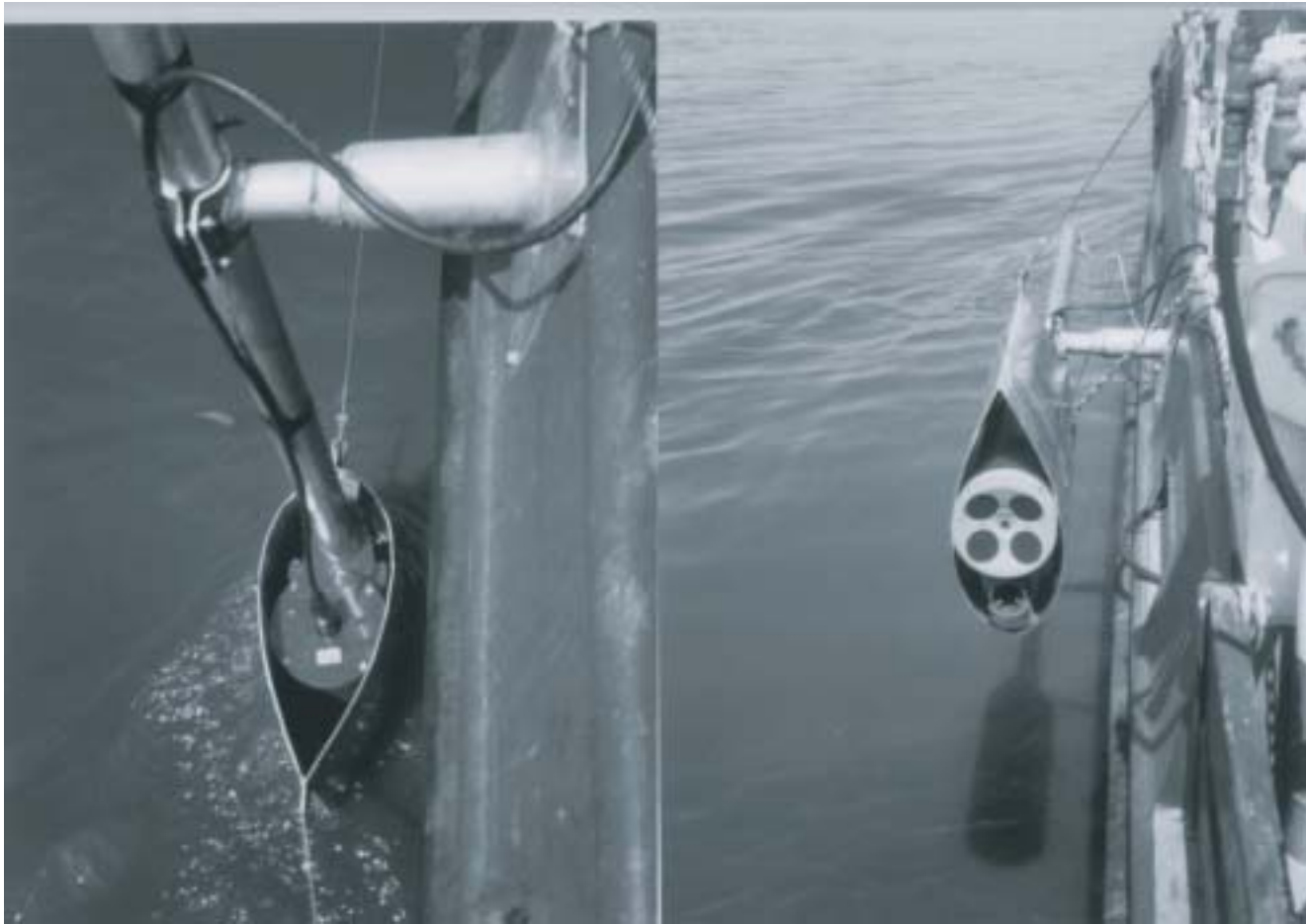
Figure 4.8. Two views of an acoustic Doppler current profiler side-swing mount on a 30-meter (95-foot) vessel.
