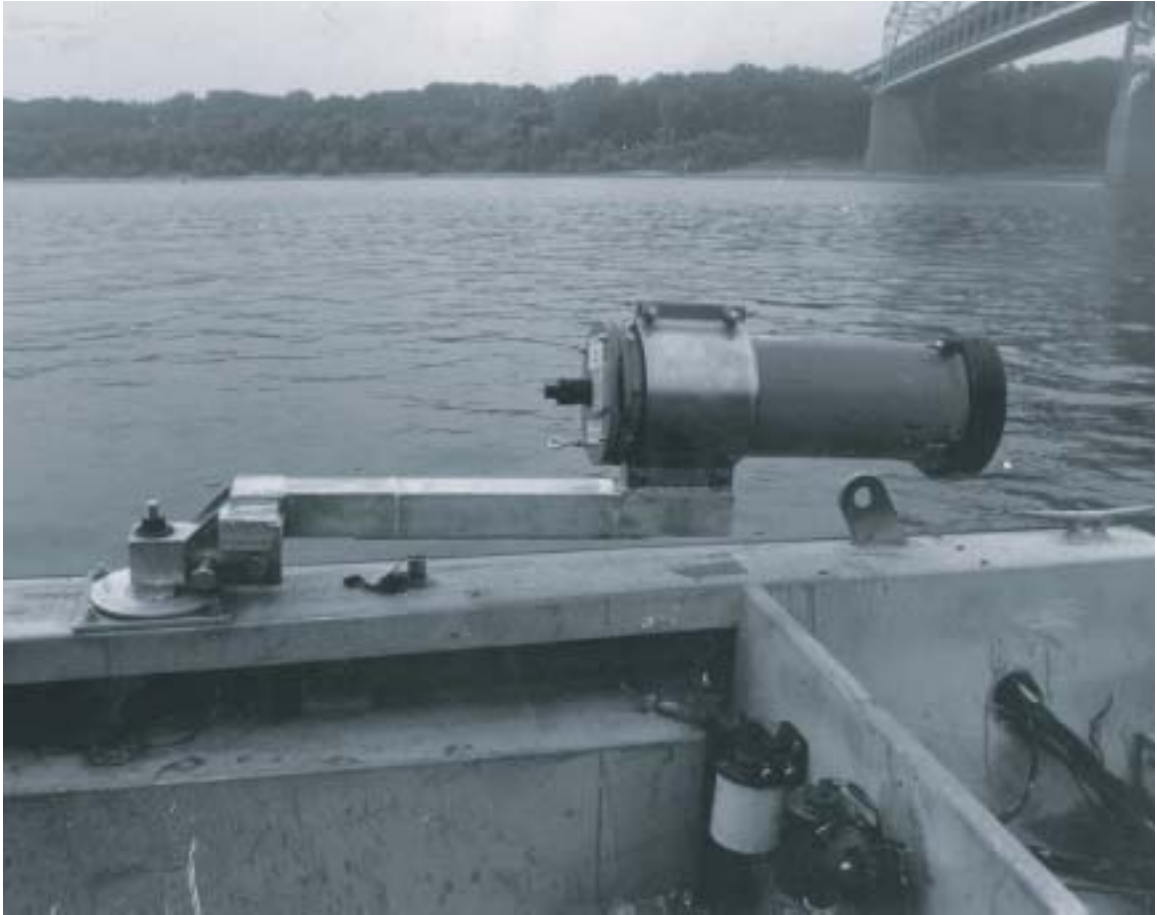
Figure 4.19. “Toggle” mount used by the U.S. Geological Survey Kentucky District.
