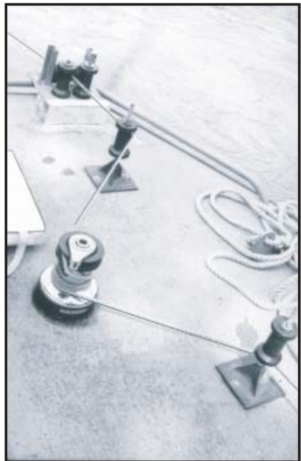
Figure 7.8. Winching system used to move an acoustic Doppler current profiler vessel at slow speeds.
