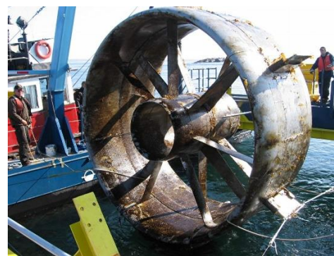
Figure 2 Fouling after 6 month (Clean Current Tidal Power Demonstration Project)
