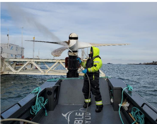
Fig. 7 SIT 4 rotor during on site cleaning
