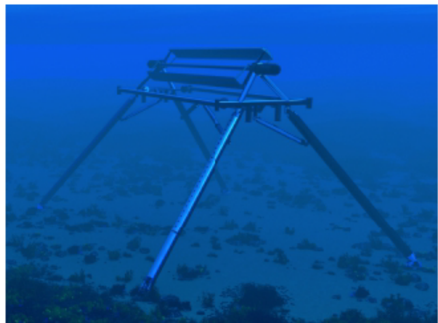
Figure 7: Cyclorotor WEC concept suggested by the Atargis Energy Corporation.
