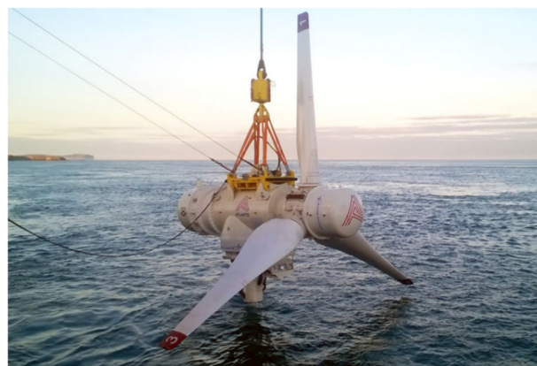
Figure 6. MeyGen tidal current power generation device. Adapted from ref. [45].
