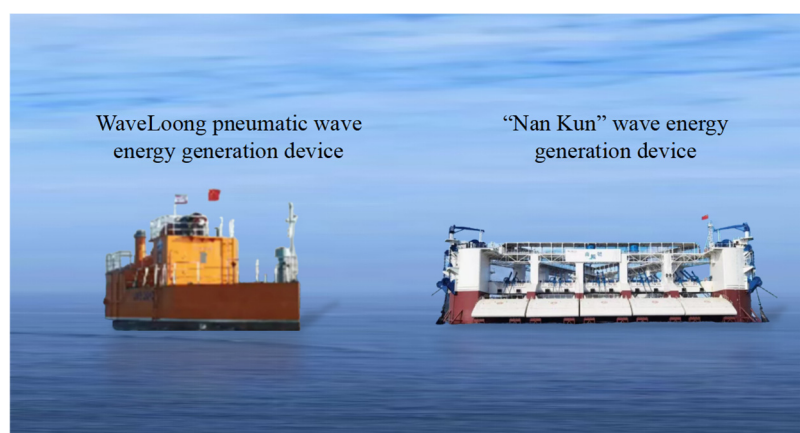
Figure 4. WaveLoong pneumatic wave energy generation device (left in the figure), “Nan Kun” wave energy generation device (right in the figure). Adapted from ref. [26].
