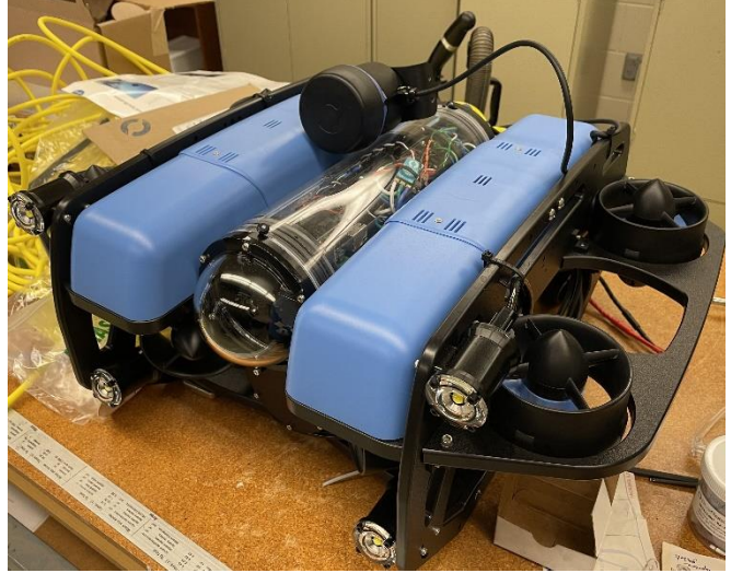
Figure 2: BlueRov2 hardware configuration.
