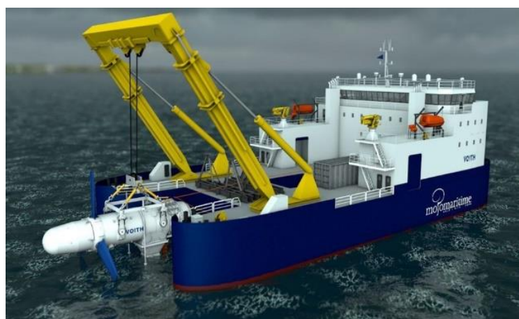
Figure 10 – The “High Flow 4” (HF4), a vessel concept designed by Mojo Maritime (now James Fisher) for supporting tidal stream projects [101].
