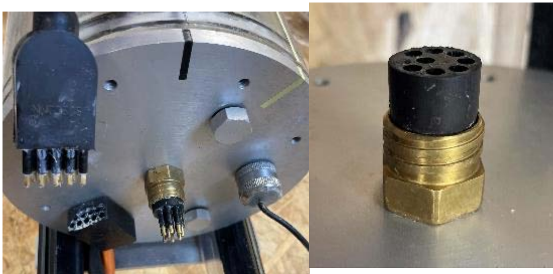
Figure 7. Electronics enclosure assembly showing Mcartney connectors opened.
