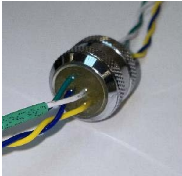
Figure 4. Combined USB (white/green) and RS485 (blue/yellow) cable penetration. The cable is potted into an off the shelf plumbing fitting with G1/4" thread and o-ring seal. See section 7.2 for further details.
