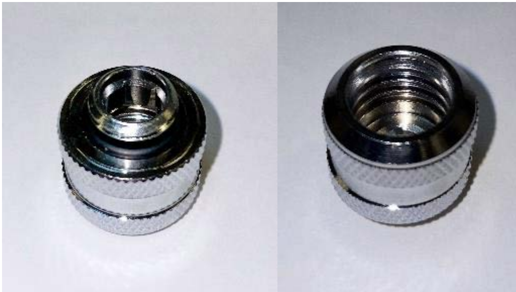
Figure 5. Picture of the G1/4" plumbing fitting used for cable penetrations. Left: external G1/4" thread with o-ring seal. Right: Internal grooves. The fitting is sold for liquid cooled computers. See section 7.2 for further details.
