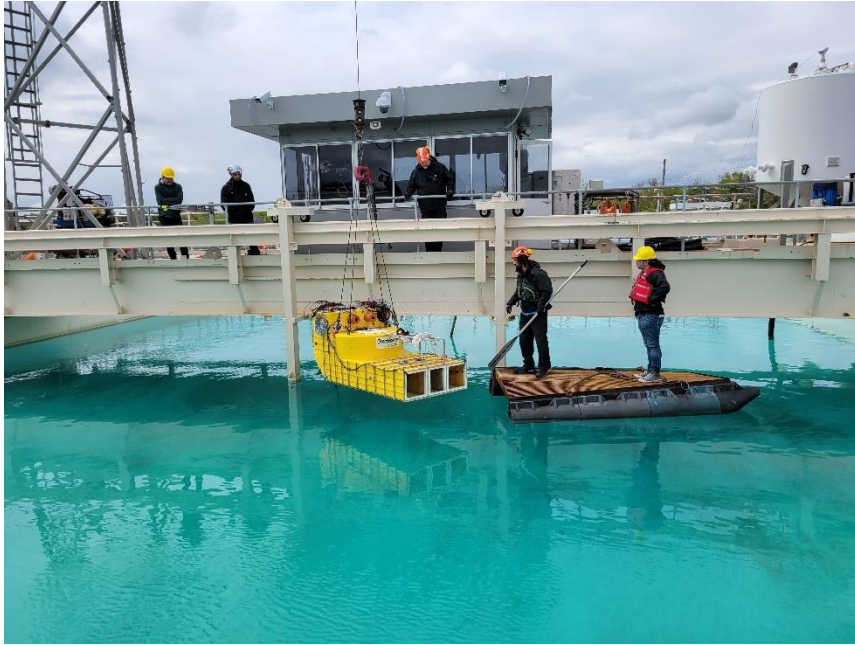
Figure 6 OE WEC model device being lowered into test tank.
