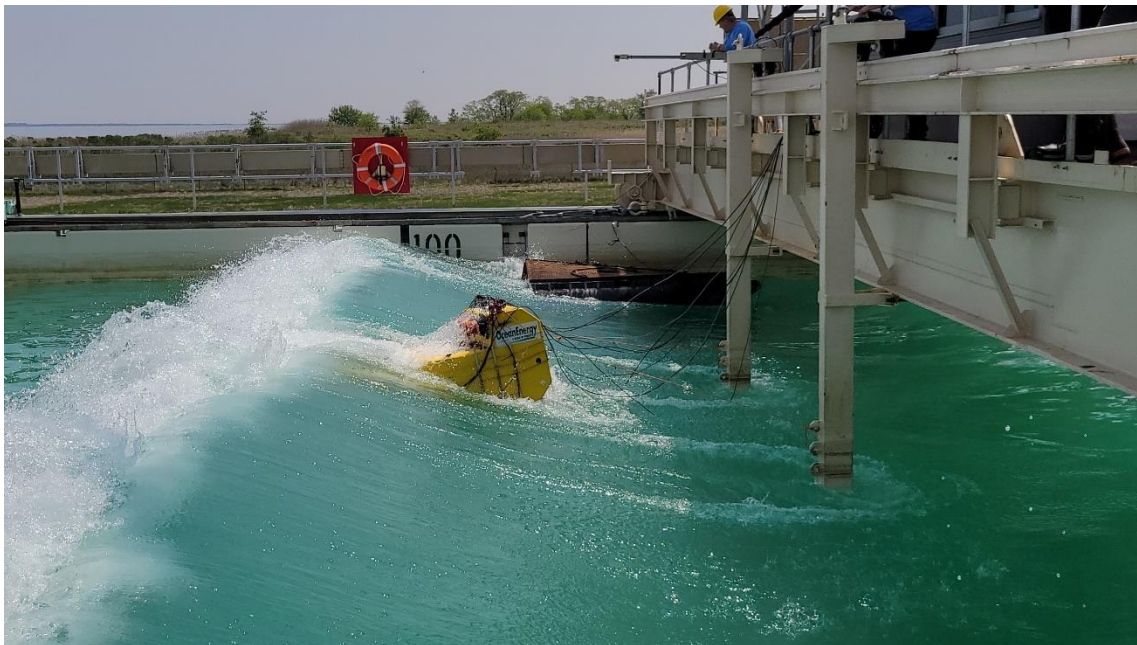
Figure 9 Example of wave tests on OE WEC model device in test tank.
