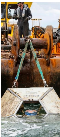
Figure 1 | EMEC ADCP in its support frame being recovered at end of Yarmouth ADCP campaign, off the Isle of Wight 2021
