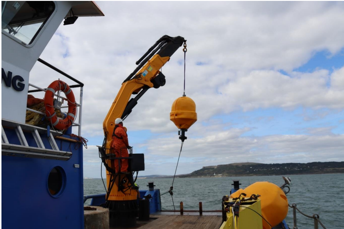
Figure 5 | Recovery of temporary vessel moorings at PTEC site used to hold vessel on station during ADCP frame recovery
