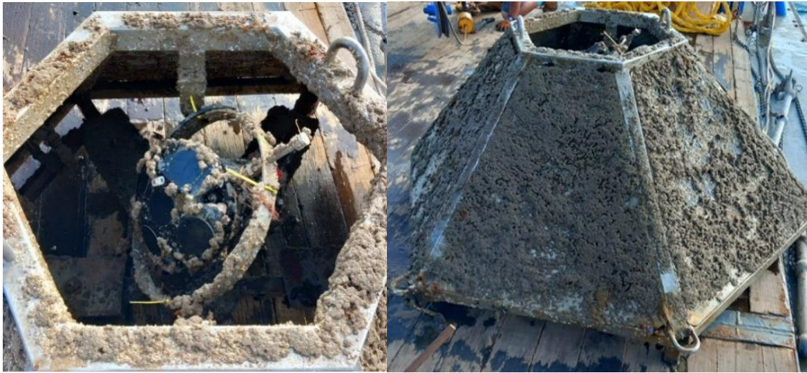
Figure 4 | ADCP upon recovery from deployment at PTEC Site off the Isle of Wight
