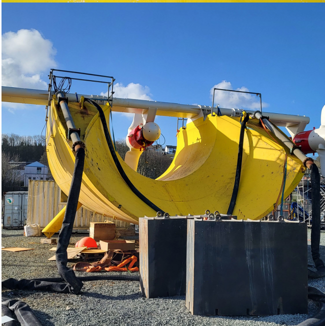
Torcado turbine blades attached to Subhub-CD platform (Credit: QED Naval)
