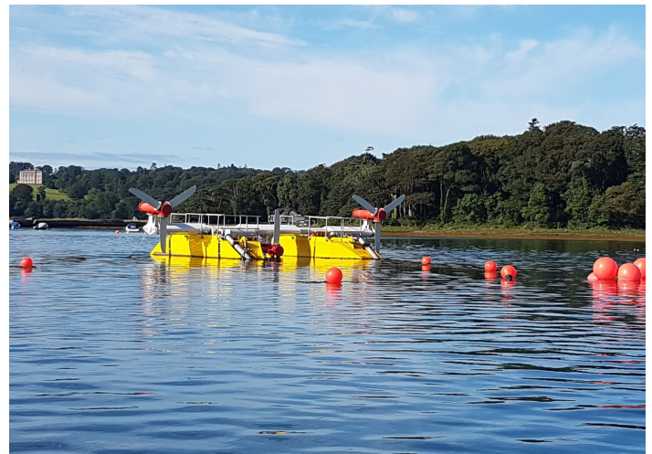
Subhub-CD turbine platform (Credit: QED Naval)
