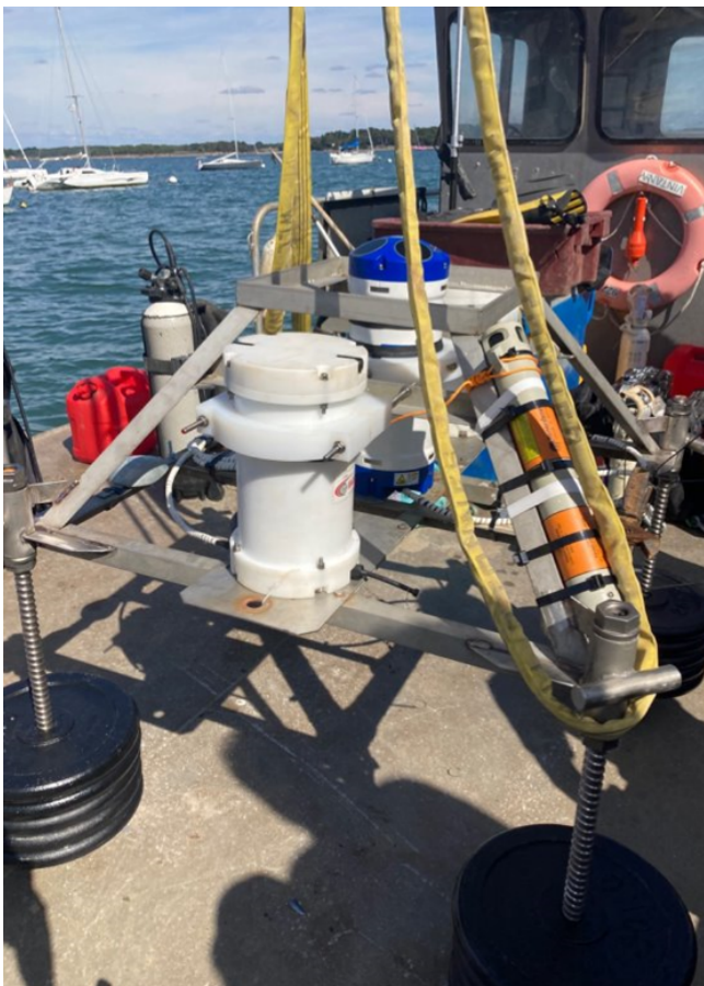
Morbihan Hydro Energies ADCP being prepared for deployment in the Golfe de Morbihan
