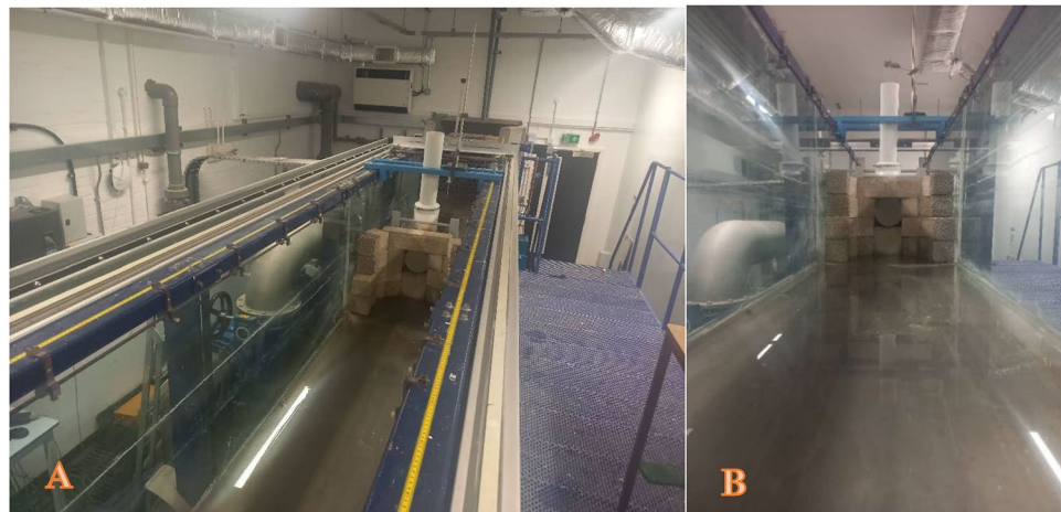
Fig. 4. Laboratory flume model used to reproduce blowhole dynamics. (A) External view of the 5 m × 0.6 m × 1.2 m wave flume. (B) Internal view showing the arrangement of concrete blocks and the assembled blowhole conduit (horizontal pipe, elbow transition, and vertical riser). Scale bar = 0.5 m.
