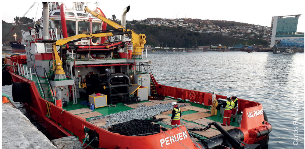
Mooring components (anchor, auxiliary buoy and chain) for MERIC's Open Sea Lab installation
