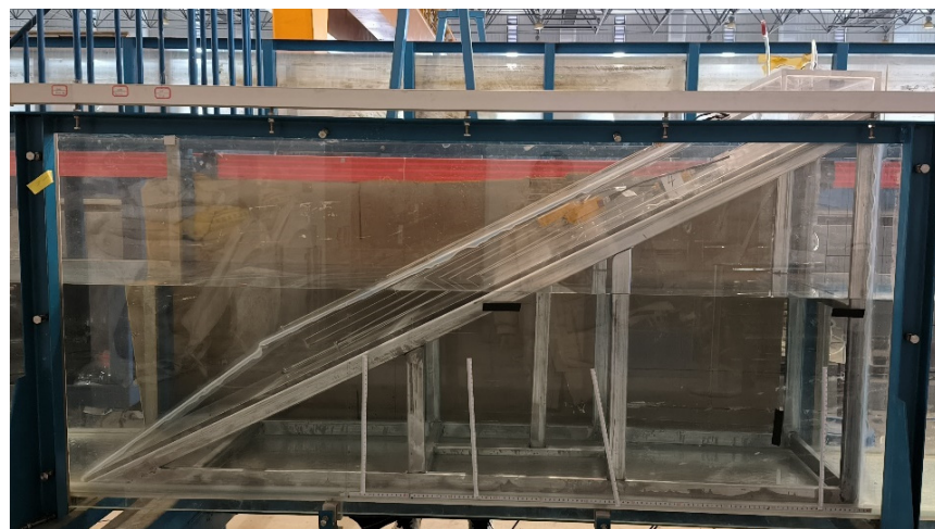
Figure 3. The OWC device in the wave flume.
