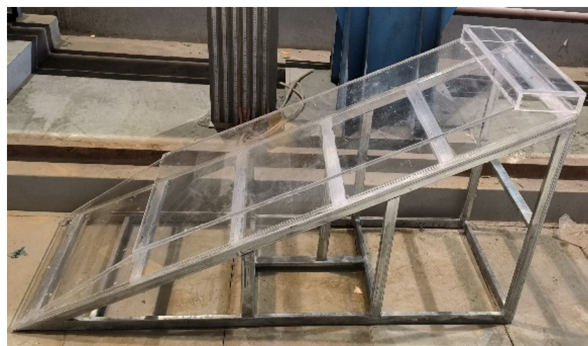
Figure 2. Physical model of the OWC device.
