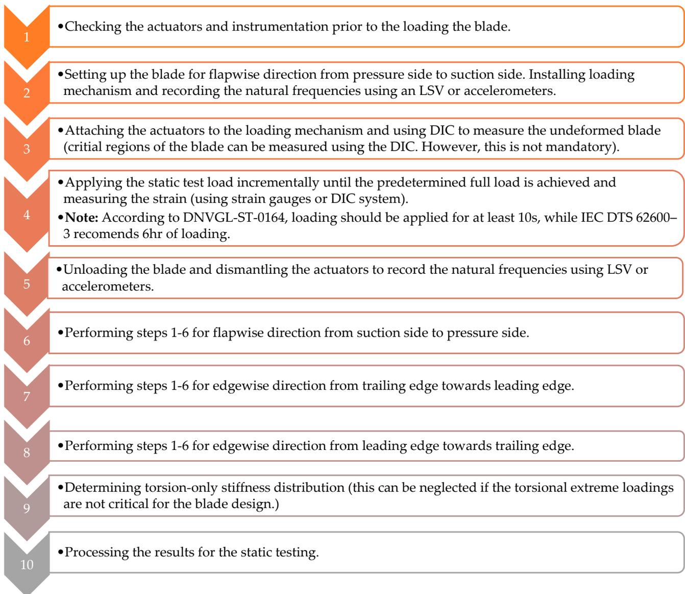
**Figure 10.** Static testing procedure for tidal turbine blades [46,47].
