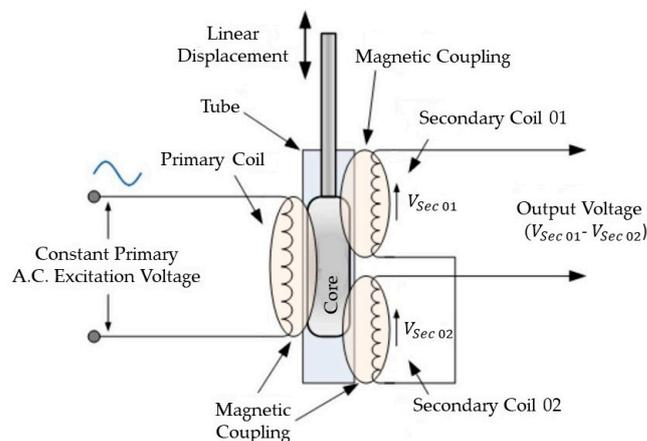
**Figure 8.** Working principles of LVDT. Obtained from [55].
