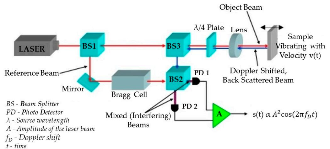
**Figure 7.** Working principles of LSV. Adapted from [54].
