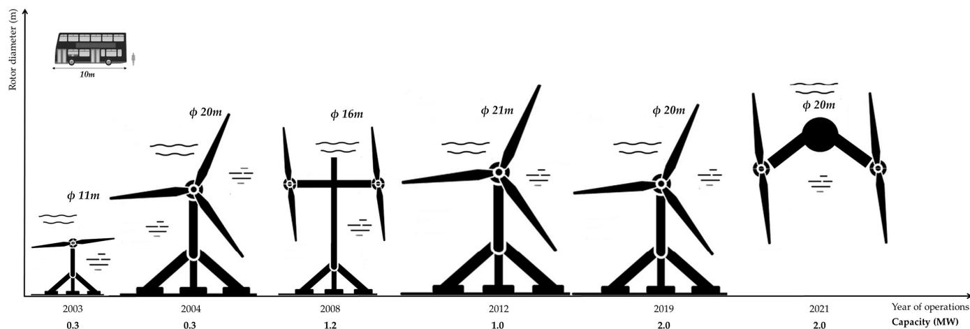
**Figure 3.** Size and capacity evaluation of tidal turbines.
