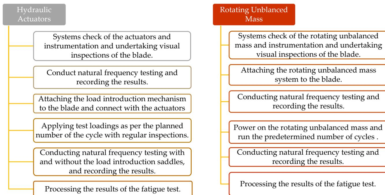
**Figure 11.** Standard fatigue testing procedure for tidal turbine blades [46,47].
