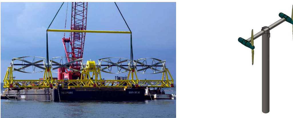
Figure 3. Ocean Renewable Power Company's beta turbine generator unit (left) and a computer rendering of the Reference Model 1 device (right).
