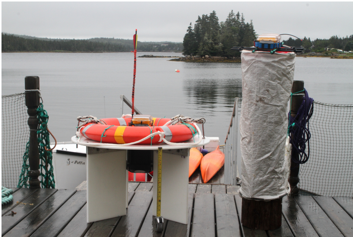
Figure 1: ADCP drifter (left) and surface flow drifter (right) - View 1. A small flag or streamer can be added to increase visibility, with consideration of maintaining minimal windage.
