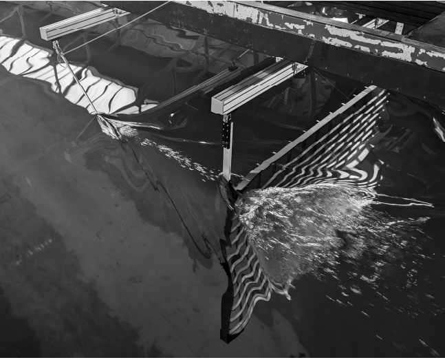
Fig. 13. Image of turbulence grid configuration C in operation in the QinetiQ towing tank.
