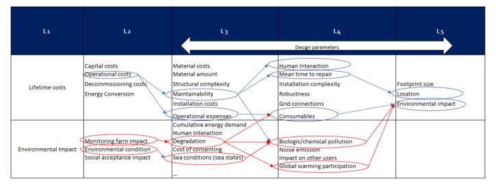
**Figure 7.** Example of using the solution hierarchy to identify relevant functional requirements from the high-level energy trilemma to meet customer requirements through specific design parameters.
