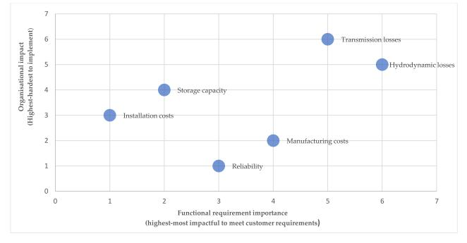
**Figure 4.** Example highlighting functional requirements with respective overall impacts and organisational capabilities. Those further to the right are more impactful to meet customer requirements, and those closest to the bottom are easiest to implement.
