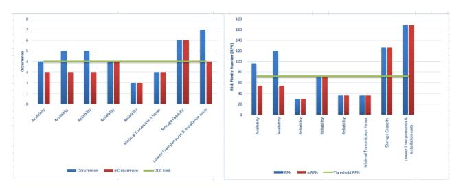
**Figure 5.** Example showing: (**left**)—the functional requirement occurrences and mitigated occurrences against occurrence limit of 4; (**right**)—RPNs and mitigated RPNs against threshold RPN of 72.
