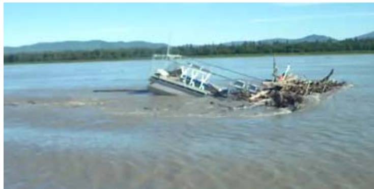
Figure 1: Debris accumulation on the 5 kW Encurrent Turbine barge in Ruby, Alaska (Johnson & Pride, 2010)
