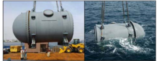
Fig. 5. Pressure test with using mock-up model
