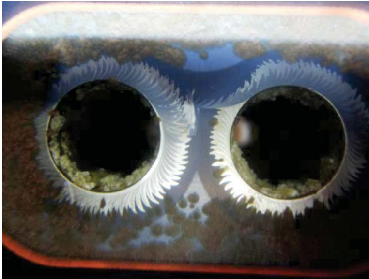
Figure 21: TFSW coupon exposed to 674m deep seawater for 1.5 years.
