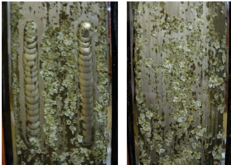
Figure 26: Images of the nitric acid baseline coupon exposed 8 months. This coupon was 3003 alloy that had undergone Chart Industries braze heating cycle.
