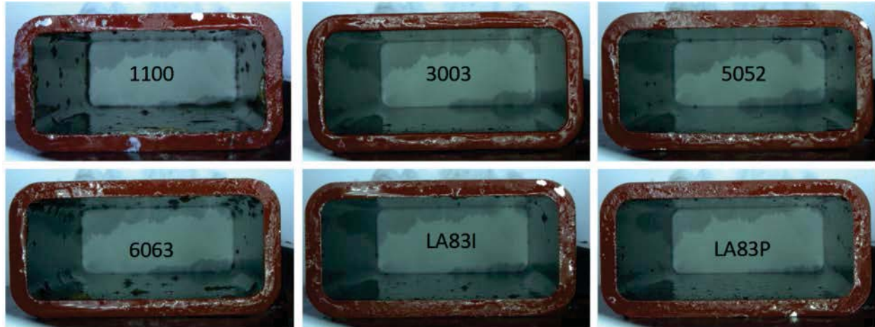
Figure 13: Representative images of the 674m deep seawater samples exposed for 3 years.
