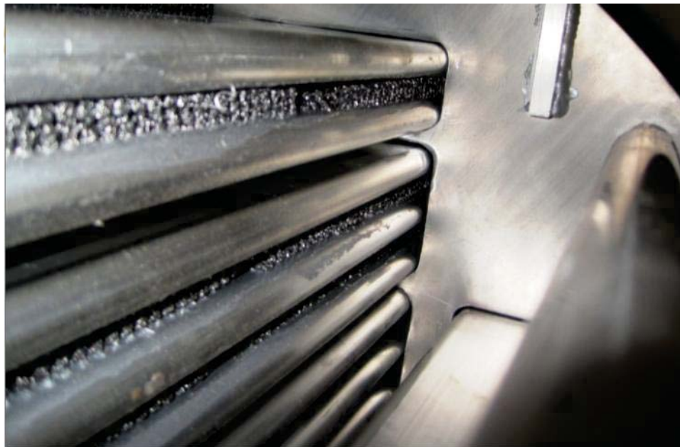
Figure 2: Graphite foam sandwiched between the multi-hollow extrusions
