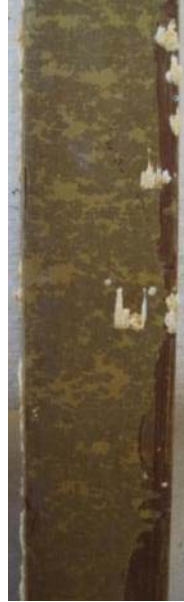
Figure 28: Siloxel coated sample after 1 year exposure in surface seawater.
