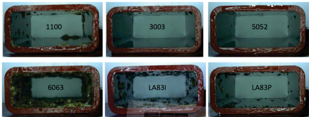
Figure 16: Representative images of the 915m deep seawater samples exposed for 3 years.
