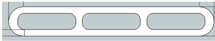
Figure 1: Multi-hollow extrusion cross section
