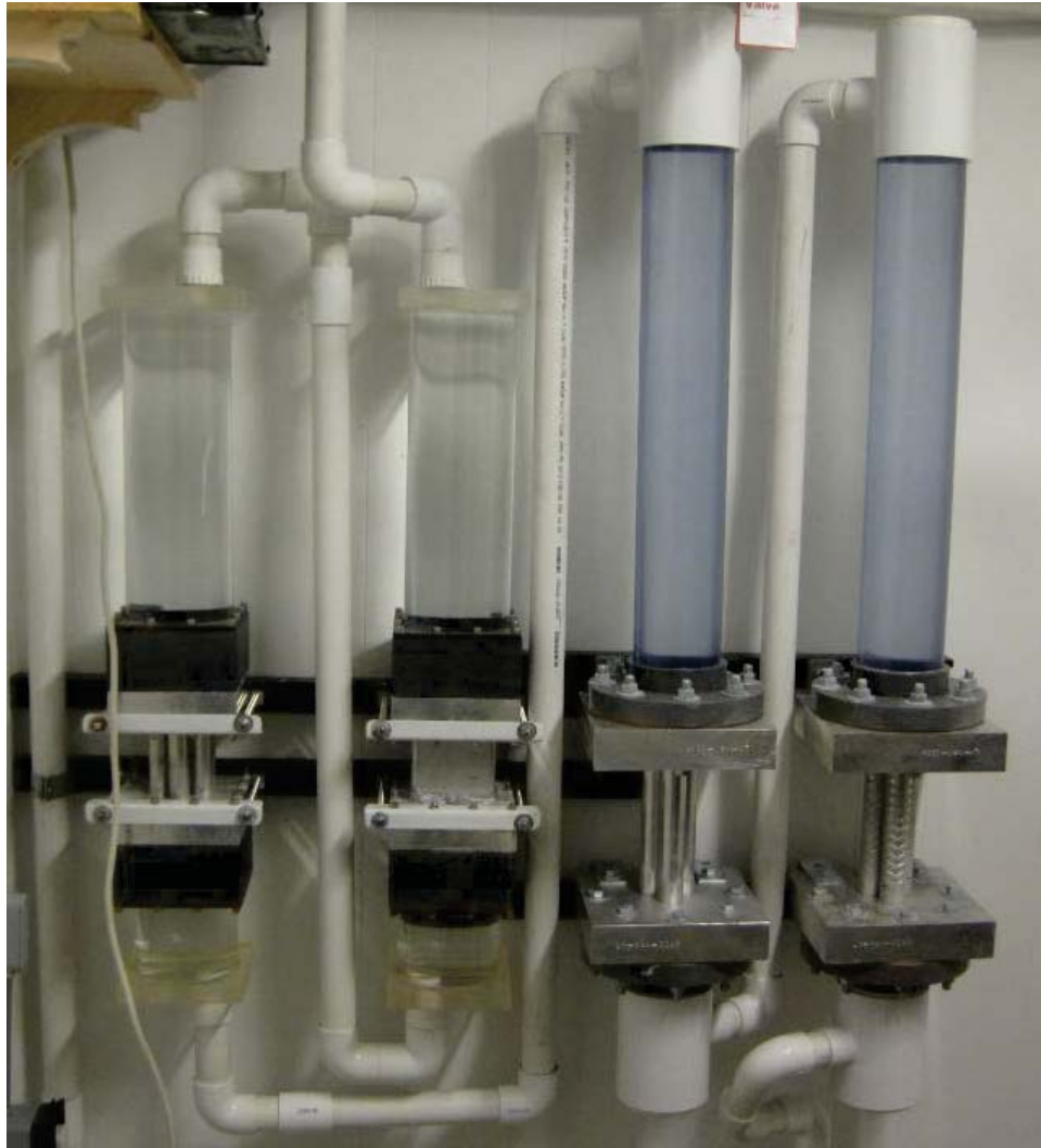
Figure 29: Multi-hollow extrusion and 3 tube coupons installed in the 674 meter deep cold seawater room.
