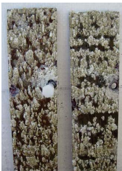
Figure 27: Comparison between the Siloxel coated sample (left) and the baseline (right) after 1 year of exposure in 674m deep seawater.
