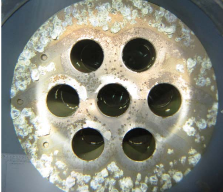
Figure 30: Expanded 7 tube water exit tube sheet after 5 months of exposure to 674m deep seawater.
