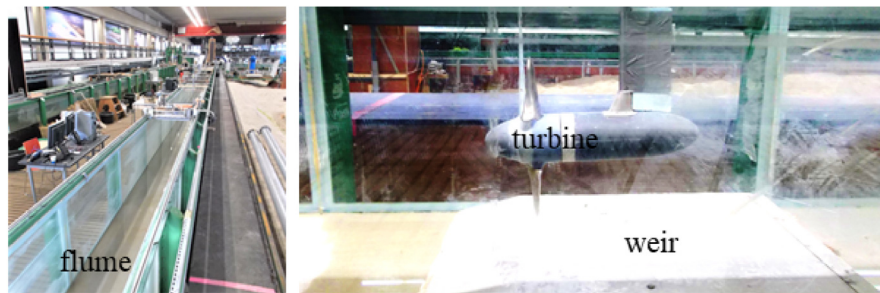
Fig. 2. Photos from the experimental set up: a) the recirculating current flume in the Laboratory of Environmental Fluid Mechanics of Delft University of Technology, The Netherlands, b) the turbine and weir; the turbine is positioned two rotor diameters upstream of the weir end in the picture ( x/D = -2 ).
