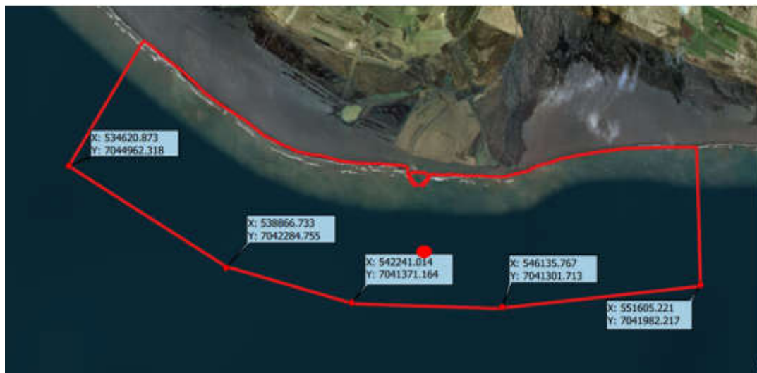
Figure 2-7 The points for which results from the regional MIKE SW wave model were extracted. The red line represents the outline of the TELEMAC model. The red dot represents the Landeyjahöfn wave buoy.
