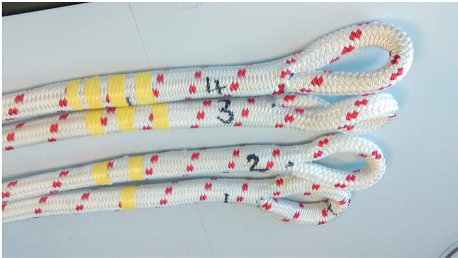
Figure 3.17: Finished eye splices of R1 (splice 1 and 2) and R2 (splice 3 and 4) specimens.
