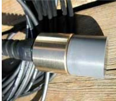
The SQ26-08 hydrophone **must be used with a recording device or preamplifier** that has a bias powered (a.k.a. plug-in powered) microphone input, and thus is included in the following **Cetacean Research**™ underwater recording systems:
