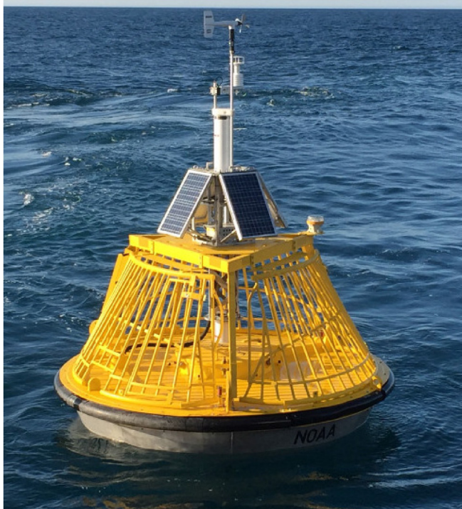
Figure 2. The picture of the US National Data Buoy Center (NDBC) 46026 station data buoy ( https://www.ndbc.noaa.gov/station_page.php?station=46026 ).
