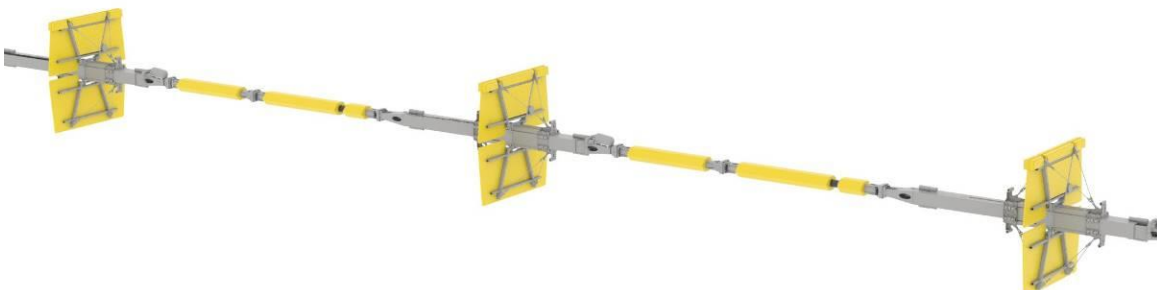
Figure 5. String of energy collectors tested with version 4. Distance between plates is 14 m.
