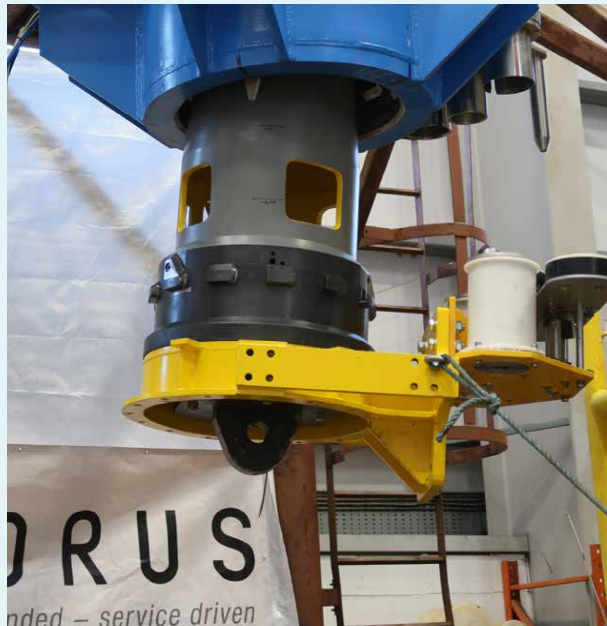
Quick Connection System (Source: Quoceant)
