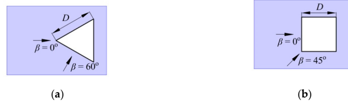
Figure 9. Two representative non-axisymmetric section profiles: (a) Equilateral triangular section; (b) square section.
