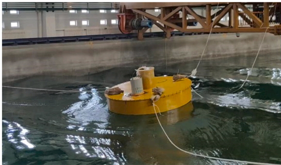
(b) Physical models of the IDWEC and buoy
