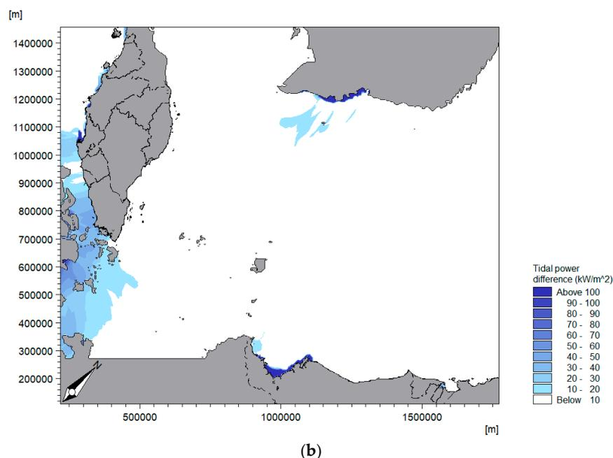
**Figure 11.** Tidal power difference with the projected sea level rise: (a) scenario 1 vs. baseline condition; (b) scenario 2 vs. baseline condition.
