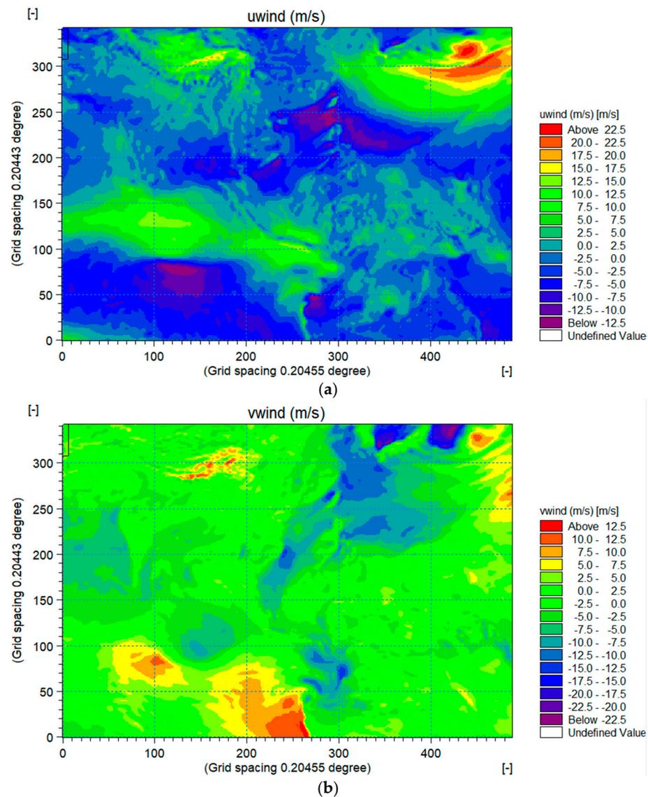
Figure 2. Wind field map: (a) u component; (b) v component.
