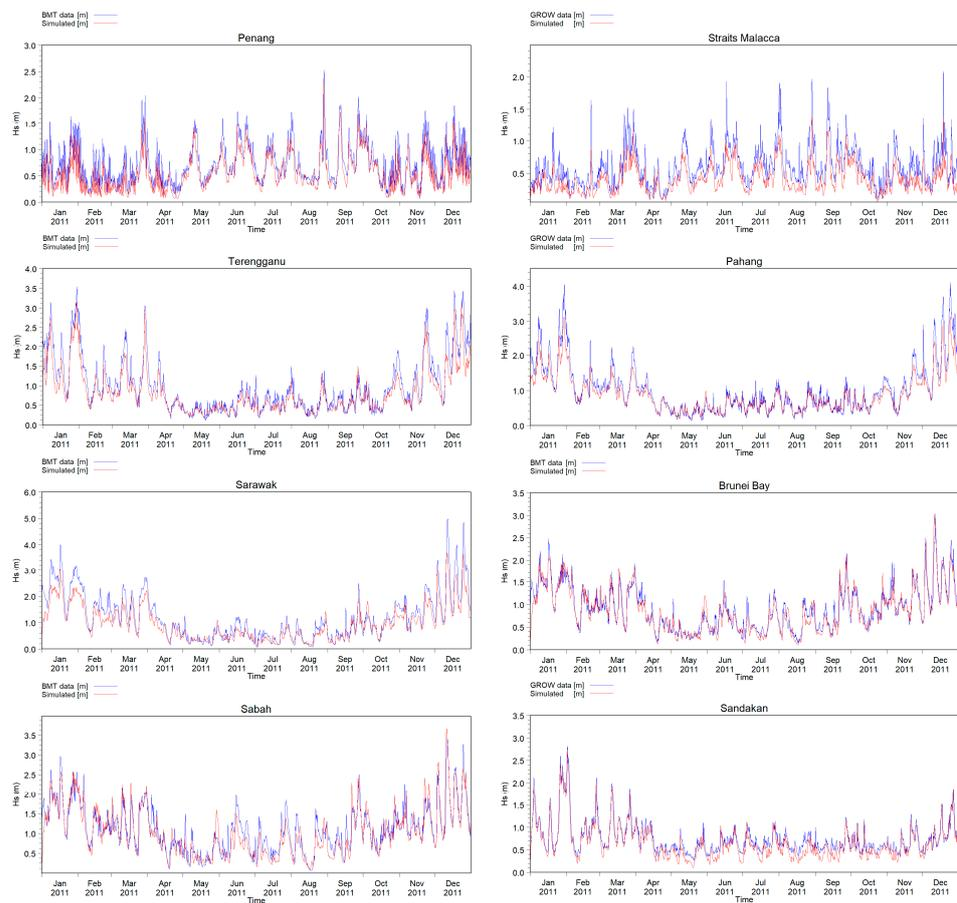
**Figure 9.** Comparison between hindcasted and simulated wave height.
