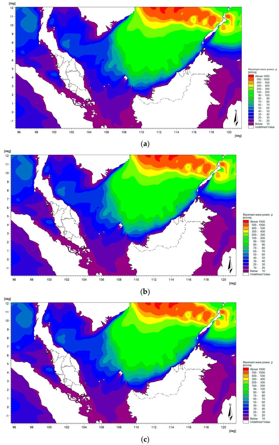
**Figure 12.** Potential location for wave energy harvesting: (a) baseline condition; (b) scenario 1 condition; (c) scenario 2 condition.
