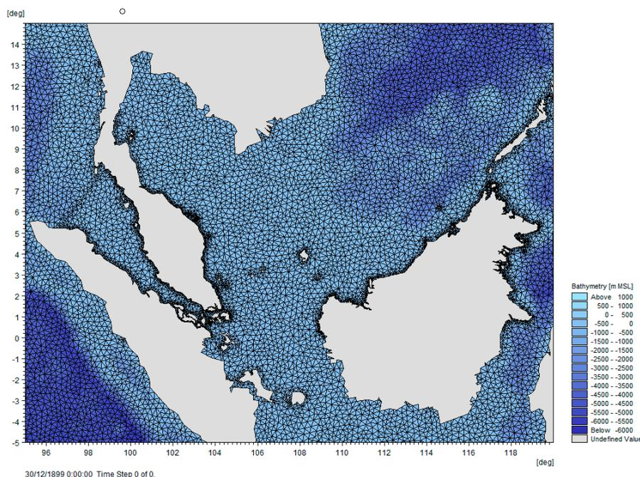
**Figure 6.** Generated mesh for wave model.
