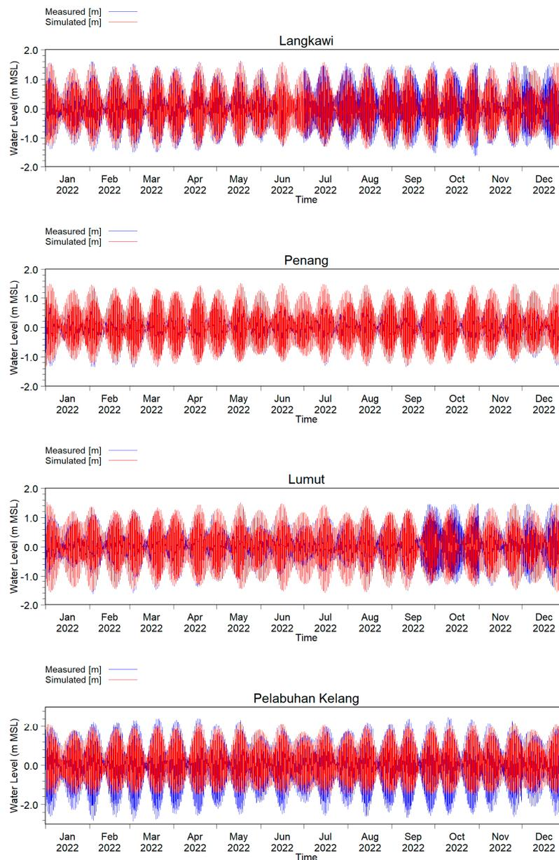
**Figure 7.** Comparison between measured and simulated water level at Langkawi, Penang, Lumut and Pelabuhan Kelang.
