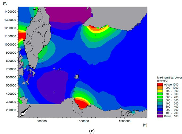
**Figure 10.** Potential location for tidal energy harvesting: (a) baseline condition; (b) scenario 1 condition; (c) scenario 2 condition.
