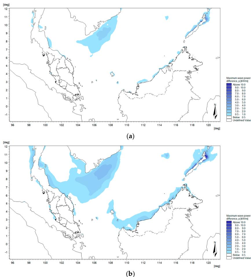
**Figure 13.** Wave power difference with the projected sea level rise: (a) scenario 1 vs. baseline condition; (b) scenario 2 vs. baseline condition.
