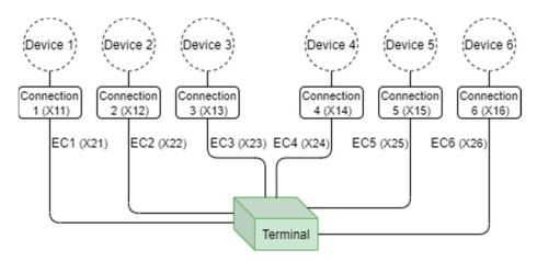
Figure 4. Schematic Illustration of Direct Topology.
