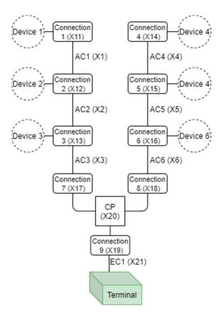
Figure 2. Schematic Illustration of Radial Topology.
