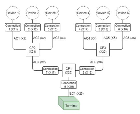
Figure 3. Schematic Illustration of Star Topology.
