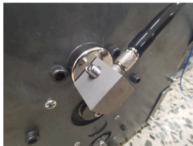
(e) ICP/IEPE piezoelectric accelerometer
