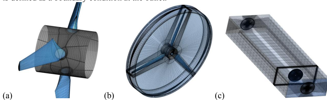
Figure 3. Mesh of the flow region (a) Blade (b) Rotor Domain (c) Stay Domain
