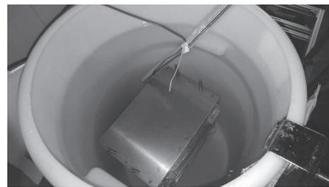
Fig. 6 Thermal energy storage unit into hot water tank.
