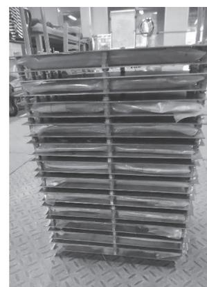
Fig. 10 Laminated thermal energy storage units (12 units).
