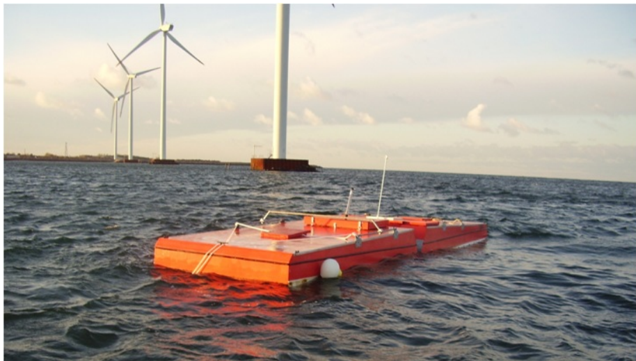
Figure 6: The 1:5 scale Crestwing device deployed off the coast of Frederikshavn Denmark from September 2011 through December 2012. This picture is courtesy of Waveenergyfyn.
