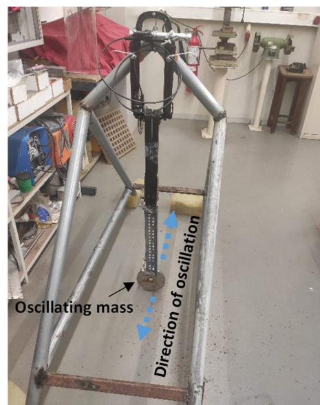
Figure 11. PTO damping calibration set-up.
