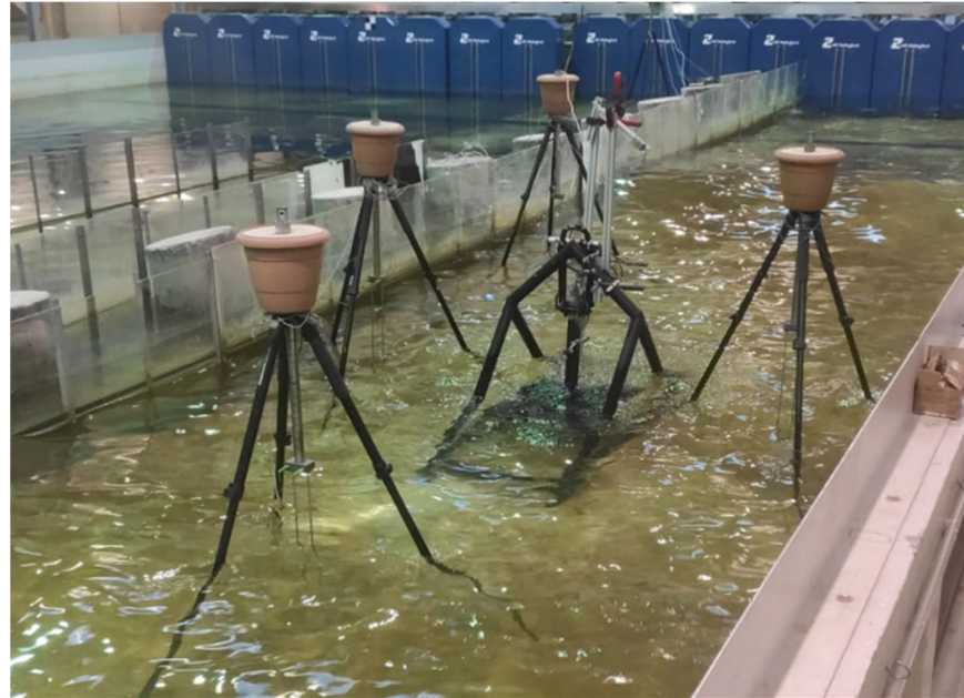
Figure 12. PWEC model during load tests and wave probes.
