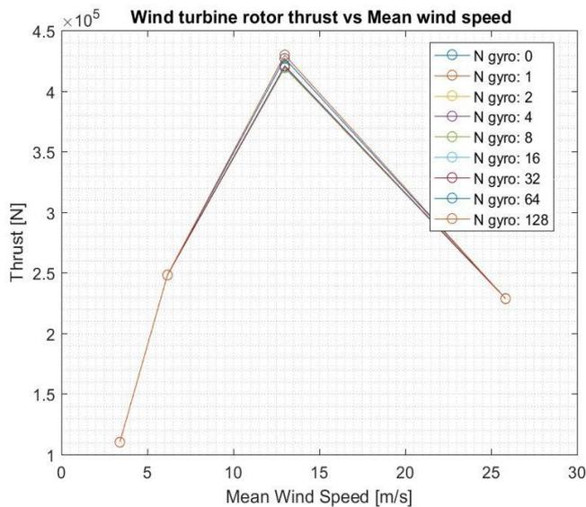
**Fig 6.** Wind turbine thrust vs mean wind speed.
