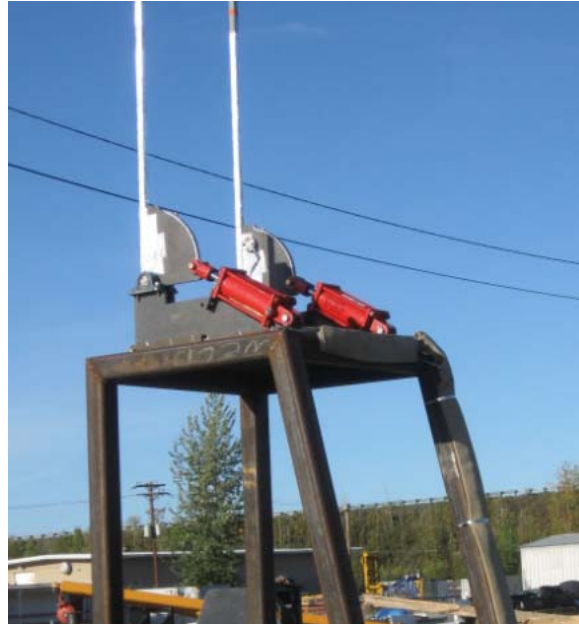
Figure 5. The mechanical debris detection device or MDDD. From Schmid 2012
