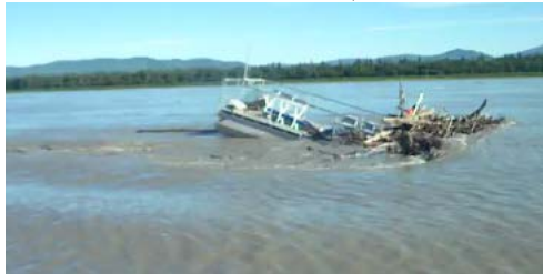
Figure 1. Debris accumulation on the bow of the 5 kW New Energy EnCurrent™ turbine barge on the Yukon River at Ruby, Alaska (from Pelunis-Messier 2010)
