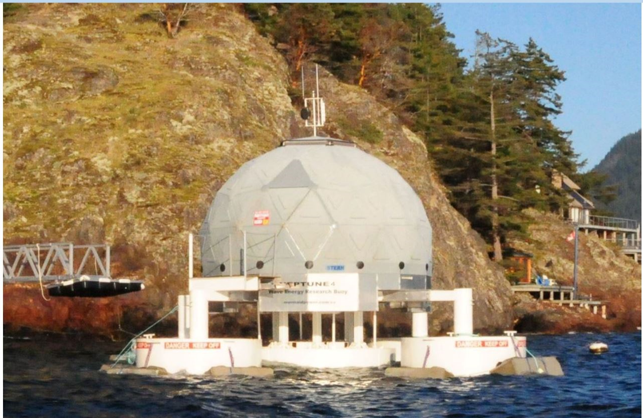
2016 Neptune 4 Dis-harmony of Floats Experiment Neptune 4 moored at Keats Island, with 35 tonne outrigger floats testing the frequency of the floating part to the motive float in waves of various sizes.
