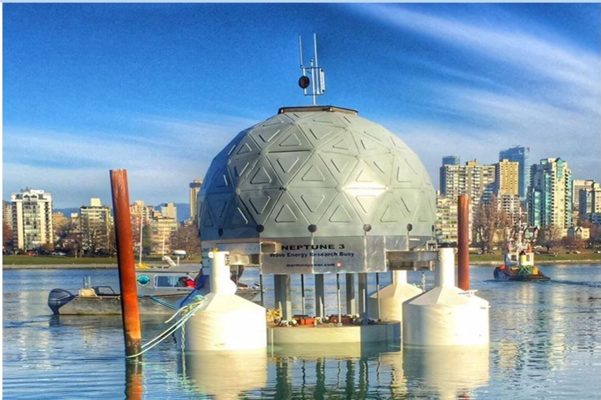
2015 Neptune 3 Shown moored at Maritime Museum, Vancouver, Tidal Compensator and electricity production from direct drive PTO-Generator tested at Keats Island.
