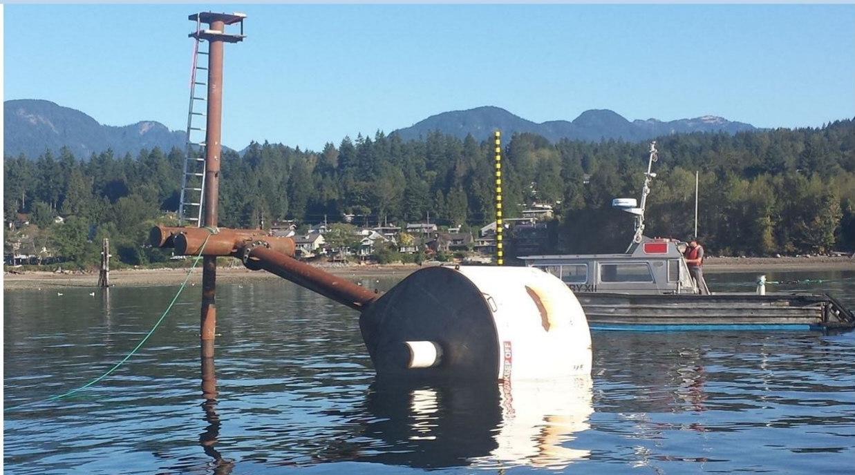
2017 Neptune 5A Test of Lever Arm Float attached to Pile to determine suitability of this approach under various conditions in various wave sizes (36 test runs), Mud Flats, Indian Arm, Vancouver Harbour.
