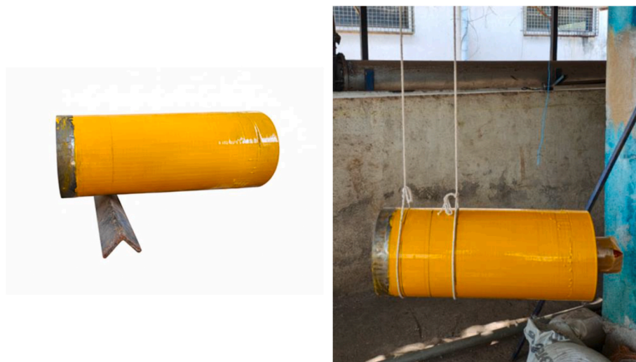
Fig. 6. (a) Suspension test and (b) bifilar test on the assembled model.
