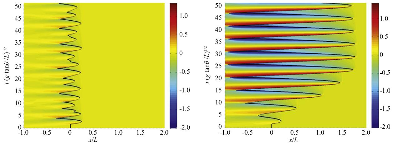
**Fig. 7.** Non-resonant (left) and resonant (right) non-dimensional velocities from a monochromatic wave on a sloping beach with slope  $\tan \theta = 0.13$  and initial shoreline at  $x = 0$  [35].  $L$  is the distance from the shoreline to the point where the bottom becomes horizontal.
