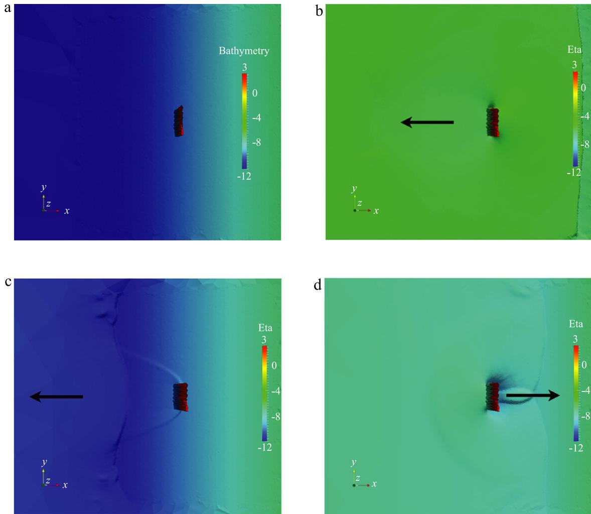
**Fig. 6.** VOLNA simulation from multiple tsunami waves hitting a 13 m high plate in an initial depth of 10 m on a sea bed with slope 0.03 (plane view). (a) Bathymetry of a fixed plate on a sloping sea bed with the shore to the right of the plate. (b) The free surface  $\eta$  after a tsunami has inundated the shore and it begins to recede. (c) 45 s later, the plate is left on dry land. (d) Another 45 s later, a subsequent wave impacts the plate.
