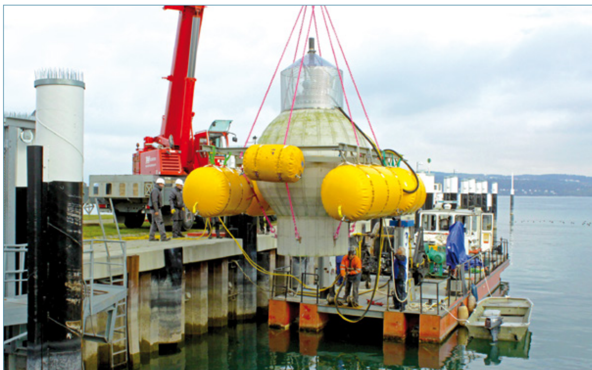
“Stored Energy in the Sea” - 1:10 scale model tested in Lake Constance, Germany
