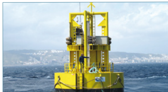
W1 wave energy device at PLOCAN test site in the Canary Islands
