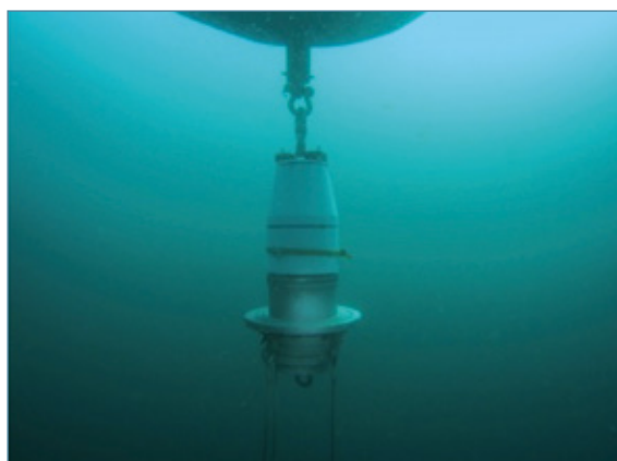
ZUNIBAL oceanographic buoy (left) and DITREL subsea connector (right) tested at BiMEP.
