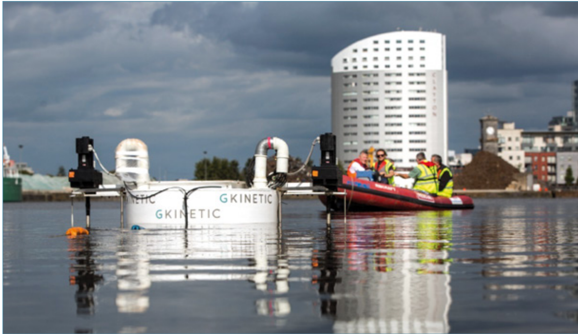
GKinetics 1:10 scale model being tested at Limerick Docks
