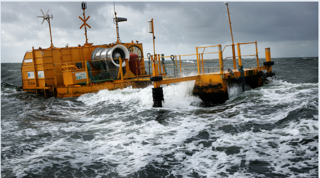
Ocean Energy's wave energy buoy being tested at Wave Hub off the Irish coast (Source: Ocean Energy Limited)
